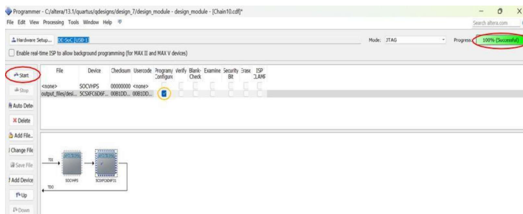
Programmer interface for programming the .sof file into the FPGA
